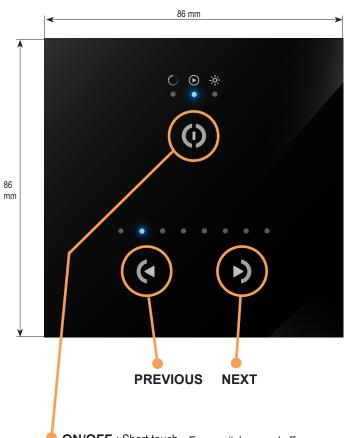
**ON/OFF** : Short touch - *Easy switch on and off* **CHANGE MODE** : Touch and hold *To switch between color, scene and dimmer mode*
